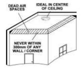
Alarms should be placed in accordance with the general guidelines shown in the diagram above. These recommendations are based on the problem of areas of "dead air" close to corners of rooms and apexes of ceilings, which could result in the prevention of heat reaching the heat detector
